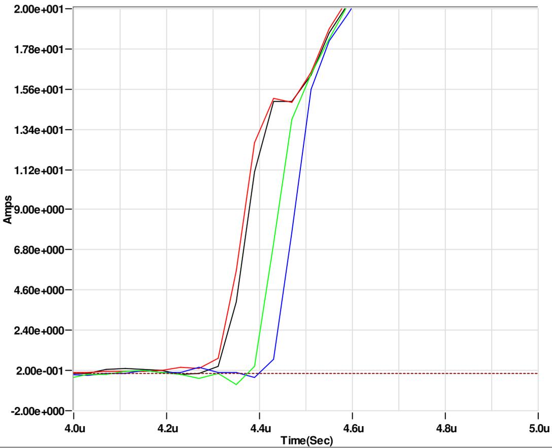
Figure 4. An example of variation in spark gap turn-on times for two 3-electrode spark gaps from manufacturer X. Vertical scale needs to be divided by 10.
