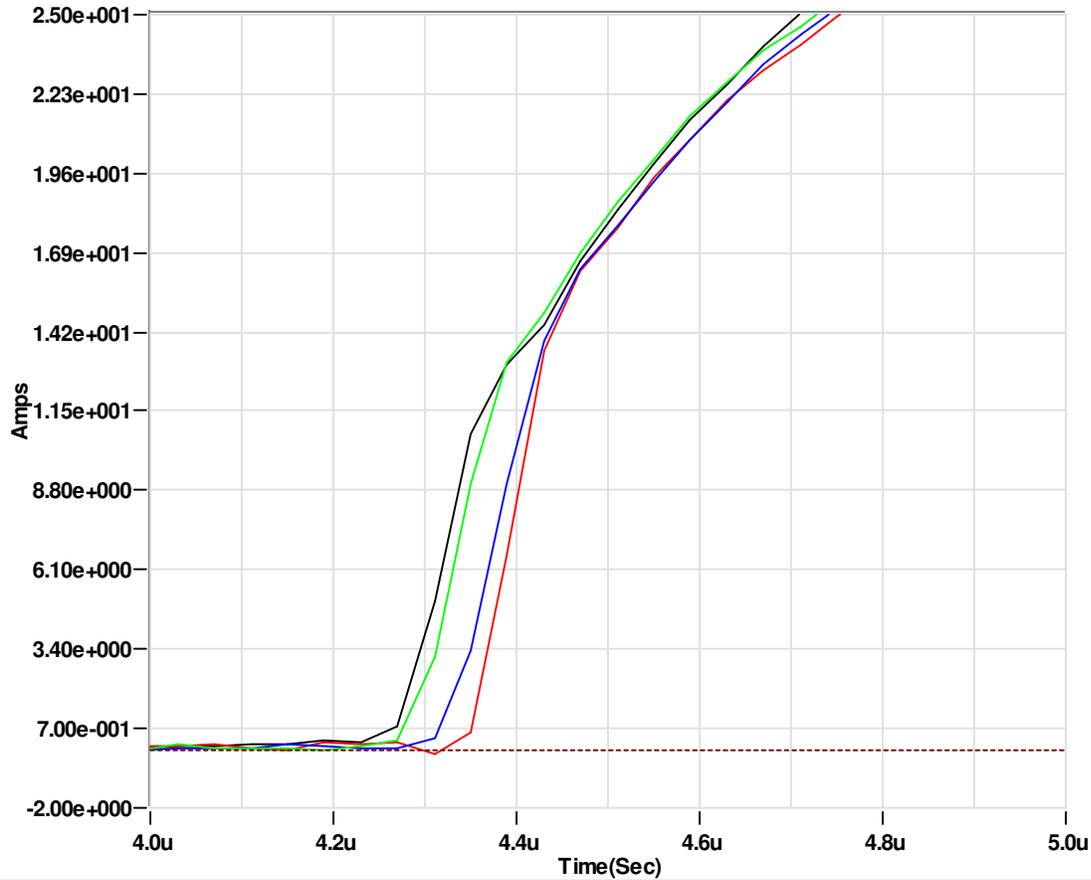
Figure 5. An example of variation in spark gap turn-on times for two 3-electrode spark gaps from manufacturer Y. Vertical scale needs to be divided by 10.
