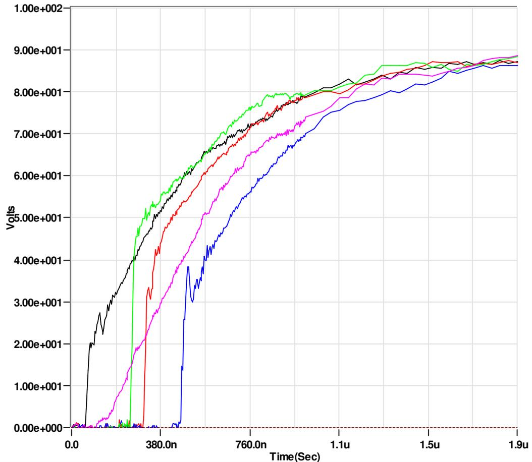
Figure 7. Comparing surge voltage delivered to a load through 4 different spark gaps from 3 different manufacturers to voltage delivered to load without spark gap present (purple trace). Note these are overlaid data taken from different oscilloscope sweeps and no inference should be made about relative turn-on times. Data are raw – vertical sensitivities have not been corrected for any differences in voltage probe gains.
