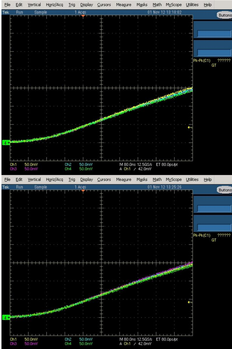
Figure 9. SCDN solid state array driven at 500 volt charge. Blue and Green pairs on top plot, Orange and Brown pairs on bottom plot. Data are raw – vertical sensitivities have not been corrected for any differences in voltage probe gains.
