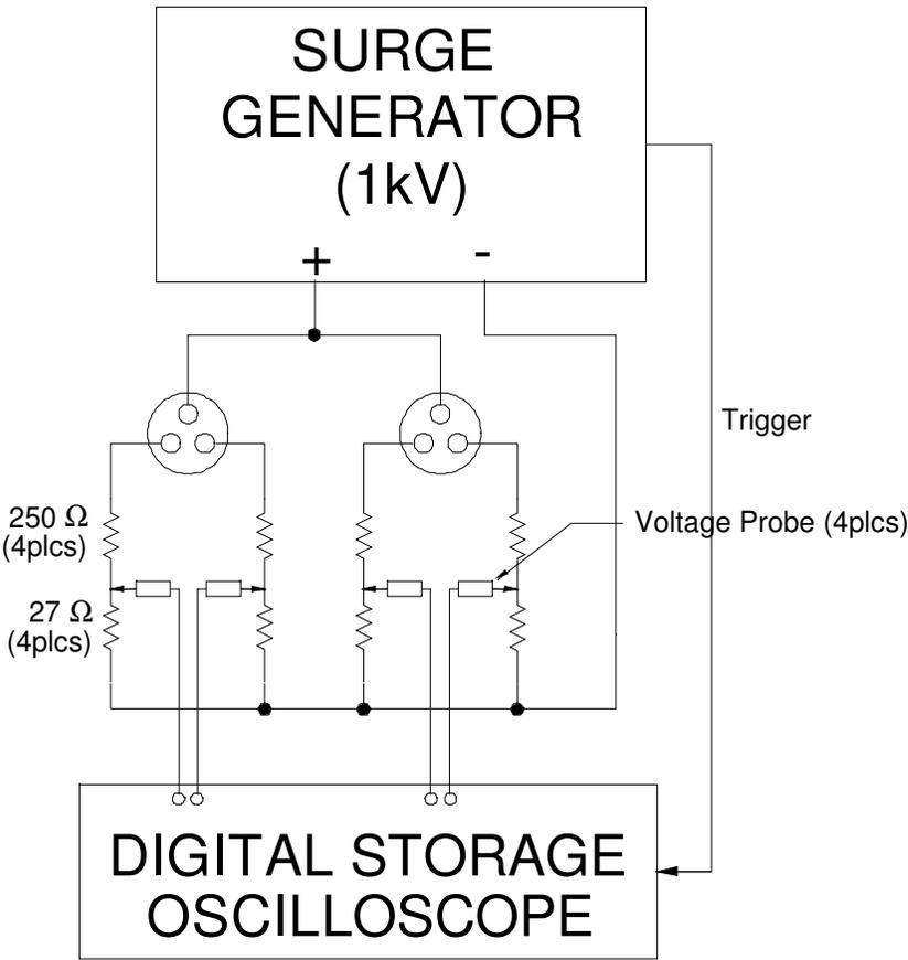
Figure 6. Test setup to compare surge voltage waveforms with and without spark gaps.
