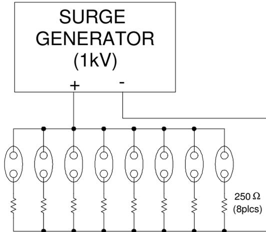
Figure 2. Test setup to investigate coupling surge using one spark gap per telecom wire.
