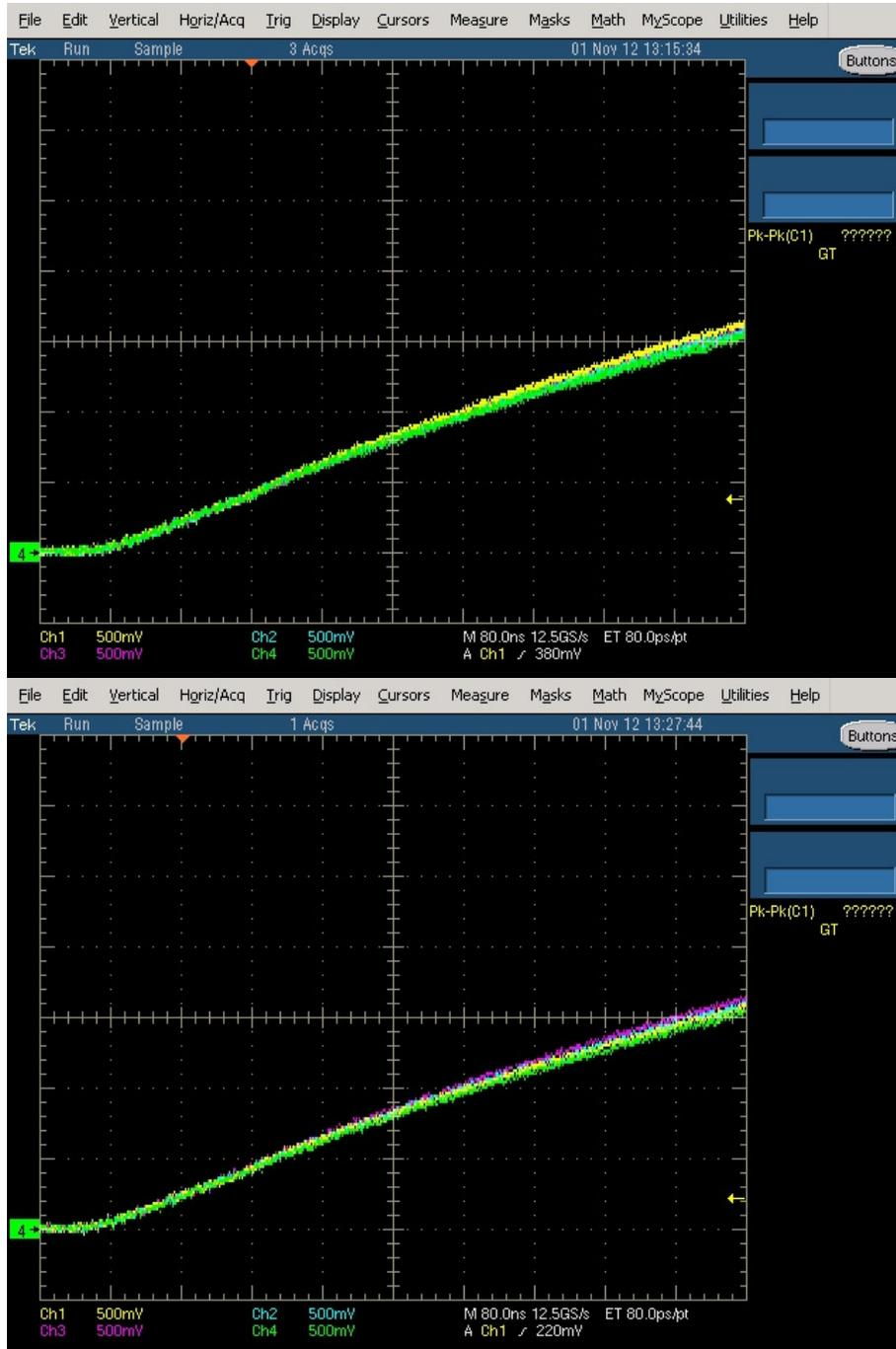
Figure 10. SCDN solid state array driven at 4000 volt charge. Blue and Green pairs on top plot, Orange and Brown pairs on bottom plot. Data are raw – vertical sensitivities have not been corrected for any differences in voltage probe gains.
