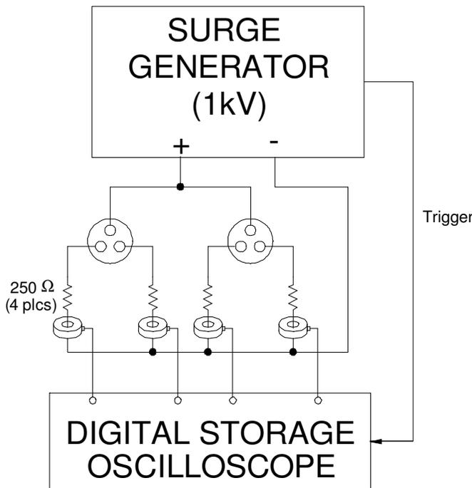
Figure 3. Test setup to investigate using one 3-electrode spark to drive a pair of telecom wires.
