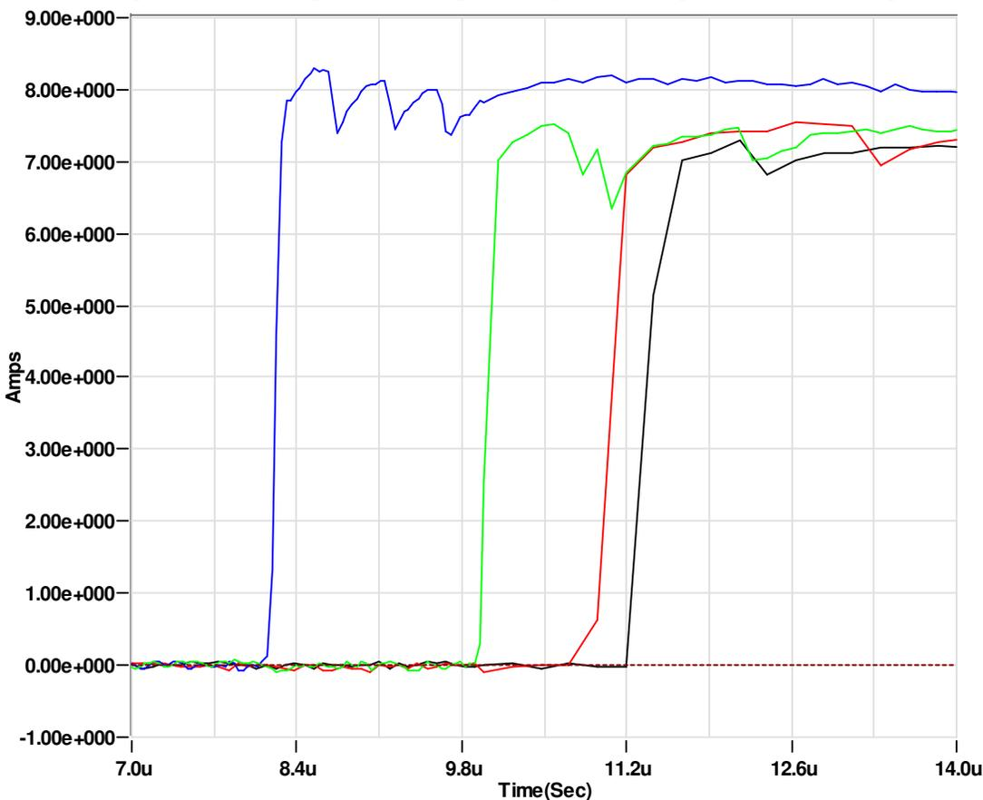
Figure 8. Example of spread in spark gap turn-on times for a 250 volt surge level for spark gaps shown in Figure 4.
