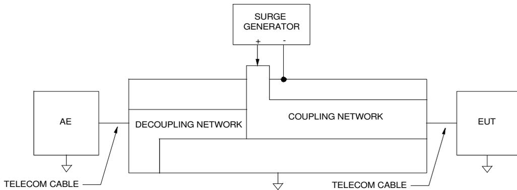
Figure 1. Generic Surge Coupling Decoupling Network (SCDN)
